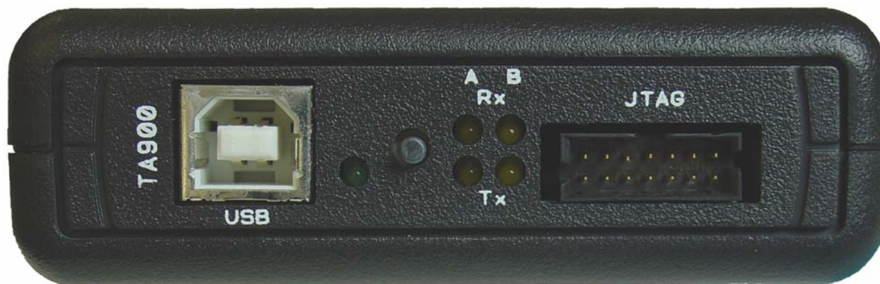
Figure 5-1 : TA900 Front I/O
