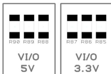
Figure 7-1 : PCI Signal Voltage Configuration Resistors (Bottom View)
