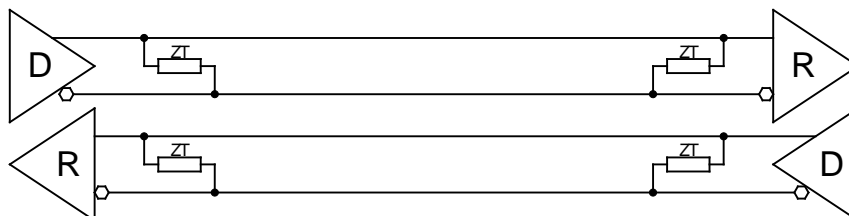
Figure 5-6 : RS485 Full Duplex Point to Point Configuration
