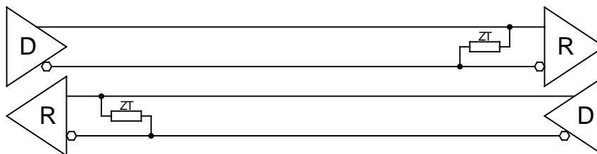
Figure 5-5: RS422 Full Duplex Point to Point Configuration
