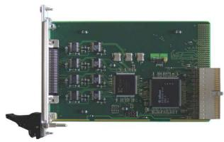
PEF 20534 An Infineon DMA Supported Serial Communication Controller (DSCC4) with integrated bus master PCI interface is used.
