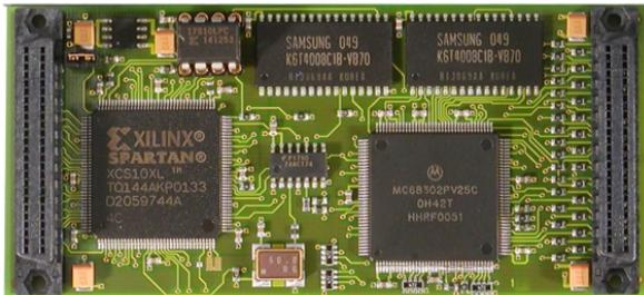
The TIP302 provides 1 Mbytes of static RAM (SRAM) as dual-port memory for both, MC68302 code and user data. The code is downloaded to the SRAM by the IP host CPU prior to removing the MC68302 reset signal by writing to a control register. Once the MC68302 reset signal is removed, the MC68302 starts fetching code from the SRAM.
