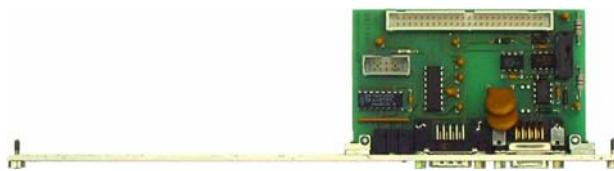
The TIP811-TM-10 transition module is required for the TIP811. It provides the optically isolated INTERBUS connector, a RS232 diagnostic port and status LED's.
