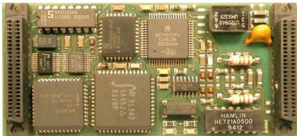
The communication is executed via a 4 Kbyte Dual Port RAM. A 32 Kbyte EPROM is used to store the protocol firmware of the NEURON Chip 3150 and the application program. All modules have a PROM with the protocol firmware and the MIP/DPR host interface software preinstalled.
