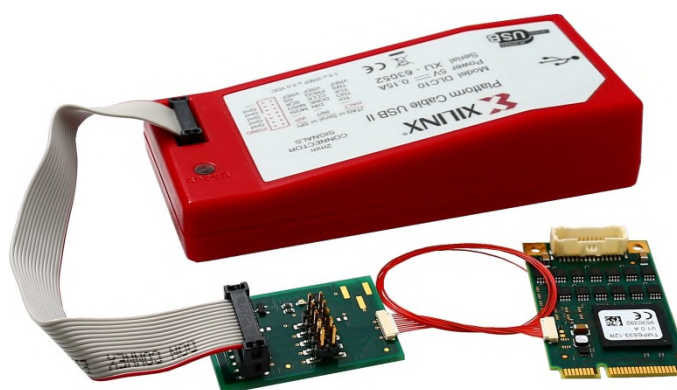
Figure 7-5: TMPE627 connected to a Programmer via TA308
