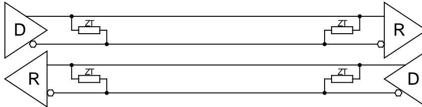
Figure 5-11: RS485 Full Duplex Point to Point Configuration
