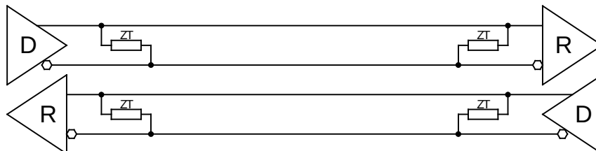
Figure 5-6: RS485 Full Duplex Point to Point Configuration
