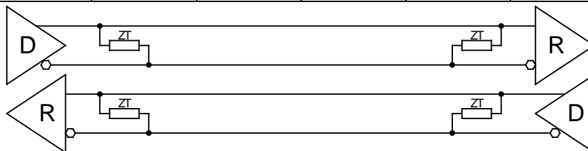
Figure 5-6: RS485 Full Duplex Point to Point Configuration
