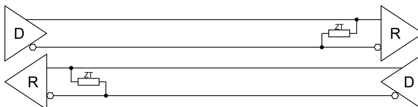
Figure 5-5 : RS422 Full Duplex Point to Point Configuration
