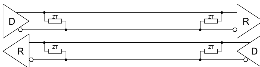
Figure 5-6 : RS485 Full Duplex Point to Point Configuration
