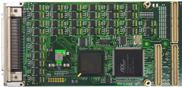
The FPGA is configured by a serial Flash. The Flash device is in-system programmable via driver software over the PCI bus. An in-circuit debugging option is available via an optionally mountable JTAG header (on the backside of the board) for readback and real-time debugging of the FPGA design (using Xilinx "ChipScope").
