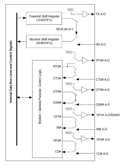
The line test contains a test of all modem lines, as you can see RTS and CTS, DTR and DSR, OP1 and RI and finally OP2 and CD. Only the static states for both electrical levels are tested on each sender – receiver line pair.
