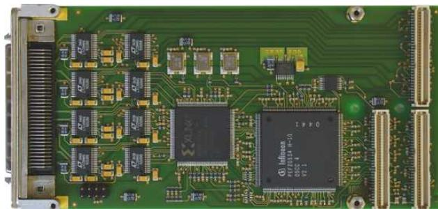
The TPMC862 provides front panel I/O via a HD68 SCSI-3 type connector and rear I/O via P14.
