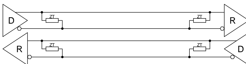
Figure 7-3 : RS485 Full Duplex Point to Point Configuration
