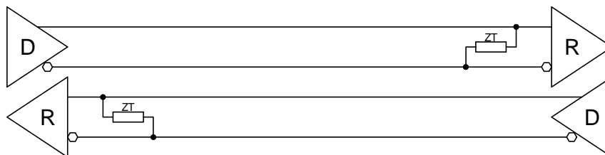
Figure 7-2 : RS422 Full Duplex Point to Point Configuration
