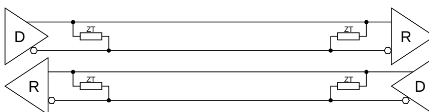
Figure 7-3 : RS485 Full Duplex Point to Point Configuration
