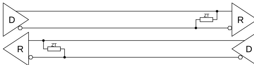
Figure 7-2 : RS422 Full Duplex Point to Point Configuration
