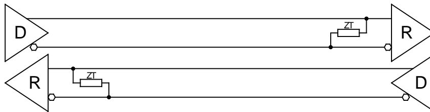
Figure 5-5 : RS422 Full Duplex Point to Point Configuration
