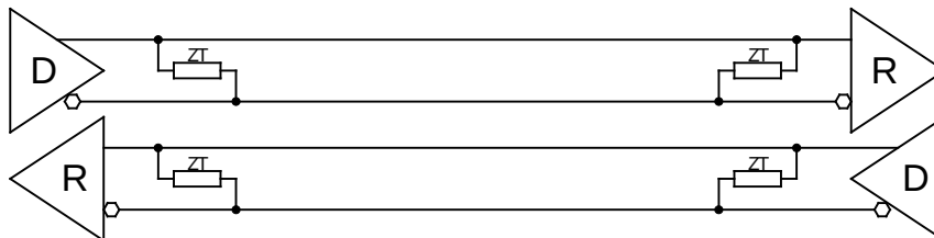
Figure 5-6 : RS485 Full Duplex Point to Point Configuration
