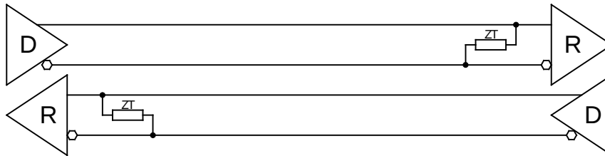
Figure 5-5 : RS422 Full Duplex Point to Point Configuration
