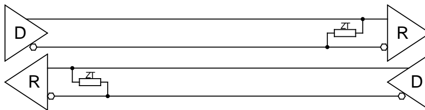
Figure 5-5 : RS422 Full Duplex Point to Point Configuration
